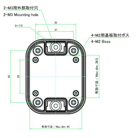
Mounting position for Pole Mounting Bracket (WPMB-M3)
